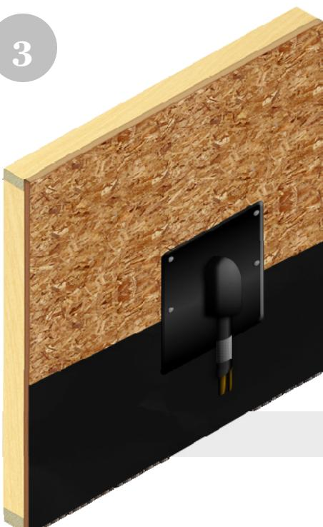
Slide the weather resistant barrier underneath the Quickflash® panel to the bottom of the line-set.
