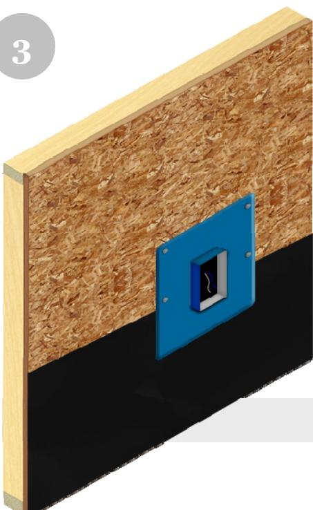
Slide the weather resistant barrier underneath the Quickflash® panel to the bottom of the electrical box.
