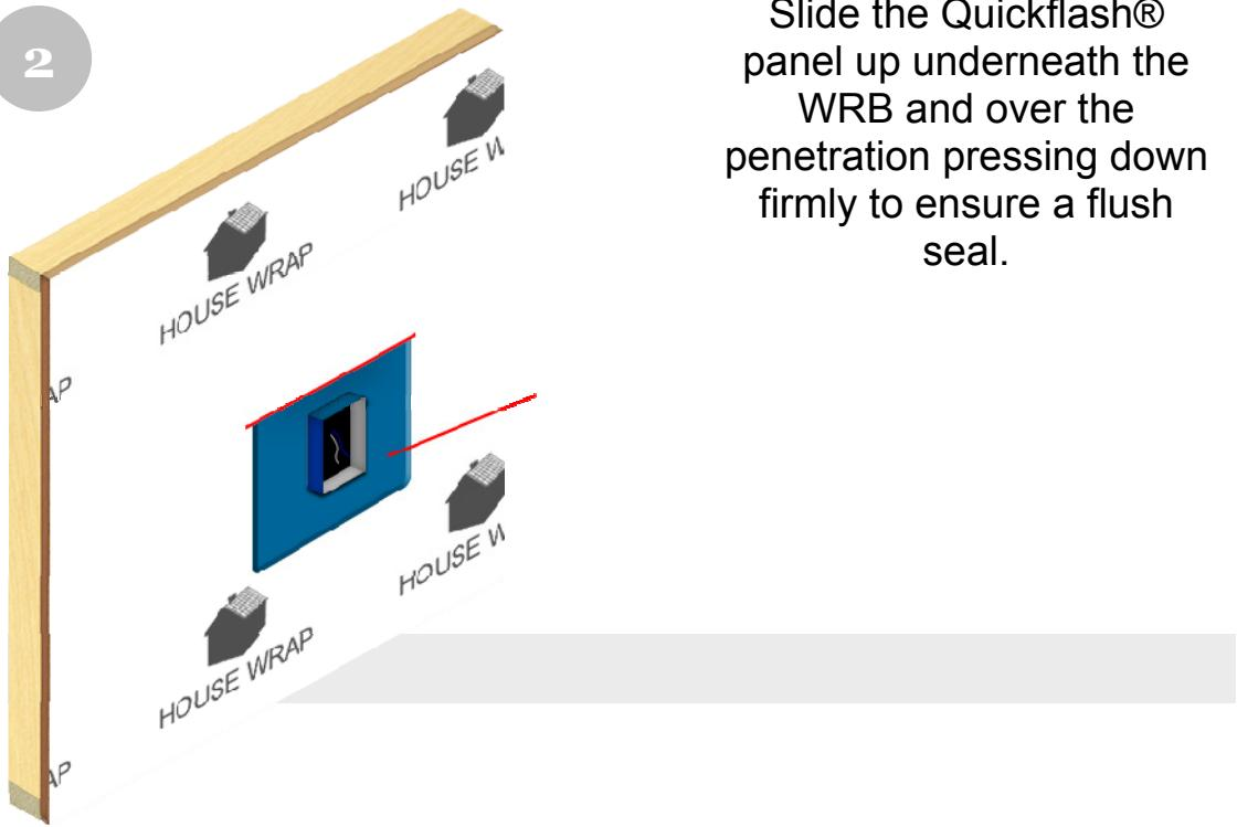
Slide the Quickflash® panel up underneath the WRB and over the penetration pressing down firmly to ensure a flush seal.
