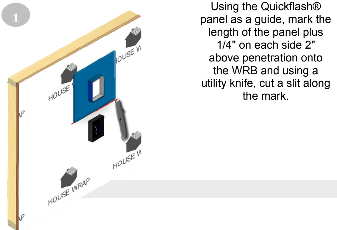
Using the Quickflash® panel as a guide, mark the length of the panel plus 1/4" on each side 2" above penetration onto the WRB and using a utility knife, cut a slit along the mark.
