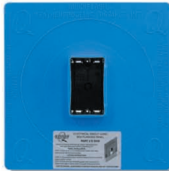
E-SGB-C 1 3/8 ELECTRICAL SINGLE GANG BOX FLASHING PANEL Used on 1-Coat Stucco & EFIS Systems. Fits Carlon Electrical Single Gang Box Only (Part # B121ADJ). 11 1/8" x 11 1/8" x 3/32" (Sold in Boxes of 12 or 24 Only)
