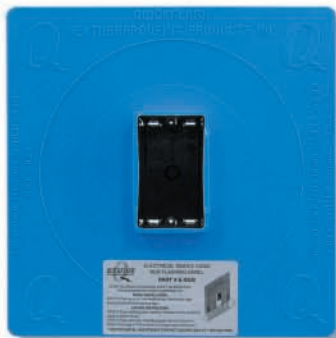
E-SGB-A 1 3/8 ELECTRICAL SINGLE GANG BOX FLASHING PANEL Used on 1-Coat Stucco & EIFS Systems. Fits Allied Moulded Electrical Single Gang Box Only (Part # 9327-N). 11 1/8" x 11 1/8" x 3/32" (Sold in Boxes of 12 or 24 Only)
