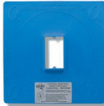
E-SGR ELECTRICAL SINGLE GANG 1/2" RAISED PLASTER RING COVER FLASHING PANEL Used on 3-Coat Stucco and Lap Siding. Fits Specified Electrical Single Gang Raised Plastic Ring Cover Only. 11 1/8" x 11 1/8" x 3/32" (Sold in Boxes of 12 or 24 Only)
