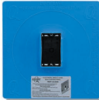
E-SGB-C 7/8 ELECTRICAL SINGLE GANG BOX FLASHING PANEL Used on 3-Coat Stucco. Fits Carlon Electrical Single Gang Box Only (Part # B121ADJ). 11 1/8" x 11 1/8" x 3/32" (Sold in Boxes of 12 or 24 Only)
